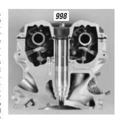
welded plastic vs. aluminum air horns on the new injection system save precious weight.
